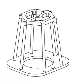
The SG123 Cage is designed to be used on the ThreadGUARD and WeldGUARD base plates as well as the SG143 Adjustable Branch Line Guard.
